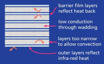
Thinsulex Silver combines a core air layer with mirrored surfaces that reflect infra-red heat. Web ultra-sonic technology joins materials without stitching which avoids air leakage or moisture contamination.
